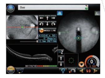
The professional mode is favored for advanced, detailed screening and analysis. In this mode, the scanning position can be adjusted to the phase fundus image and it supports capturing precise OCT images.
