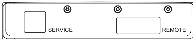
Fig. 3 Marking on left side of column (top)
