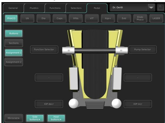
Tab. 28 Example assignment of the function buttons
